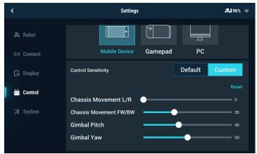
Control Sensitivity changes the signal gain that is sent to each of the component motors from the input that the operator gives through the remote controls.
