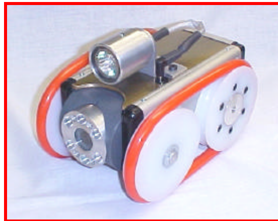
Camera Head Tilts 45° Up & 45° Down
